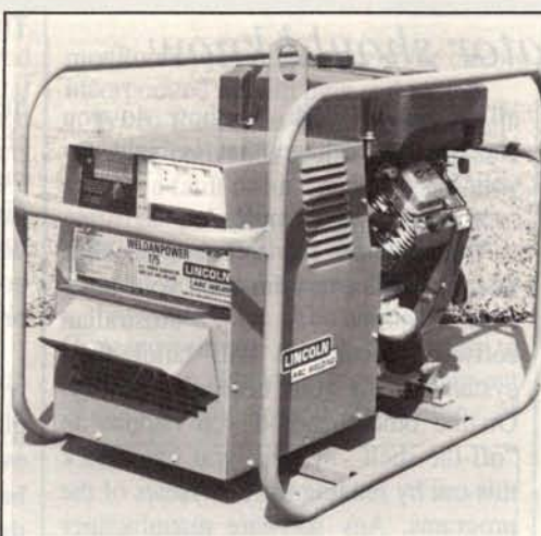
The four-stroke, two-cylinder Vanguard engine gives around 6dBA reduction in sound levels.
